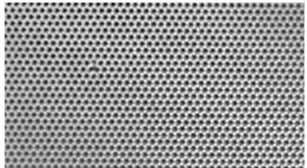
A graphene monolayer with the absence of a one single atom
